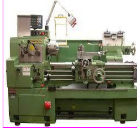
Centre Lathe - used for drilling, turning, shaping material into cylinders
